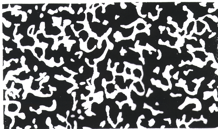
Figure 4. An image of the pore network in Vycor of mean pore diameter 50 Å, based on a transmission electron micrograph (from [50], used with permission).
